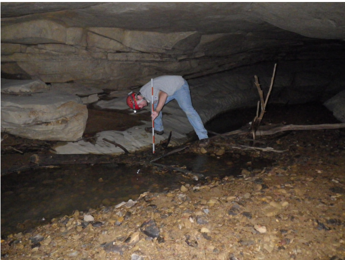
Figure 12. Chad Rigsby measuring depths across each station, to aid in calculating discharge [HH].
