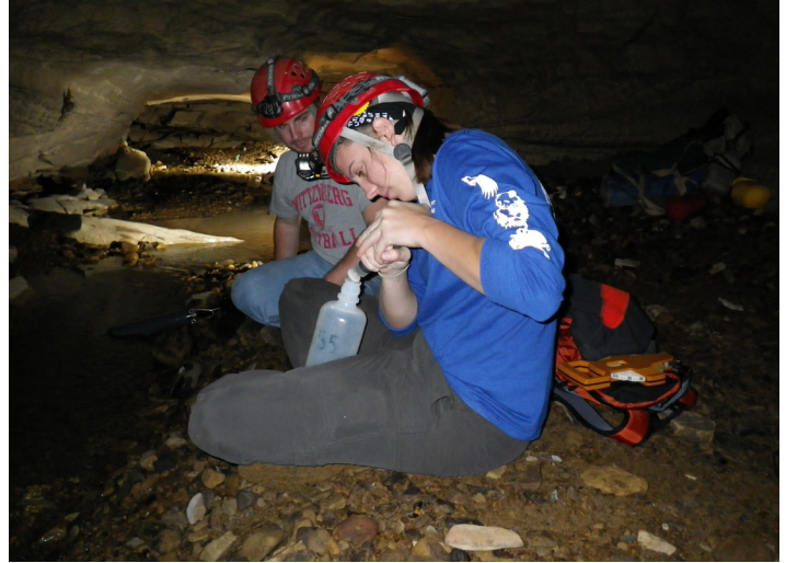
Figure 8. Kristen Shearer and Chad Rigsby filtering a water sample, to be analyzed later for background chemical levels [HH].
